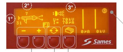
Screen« B » = Shows your own settings in one of the preselected programs (P1 to P9) Injection and dilution air and selection of a preset (U/I) package.
